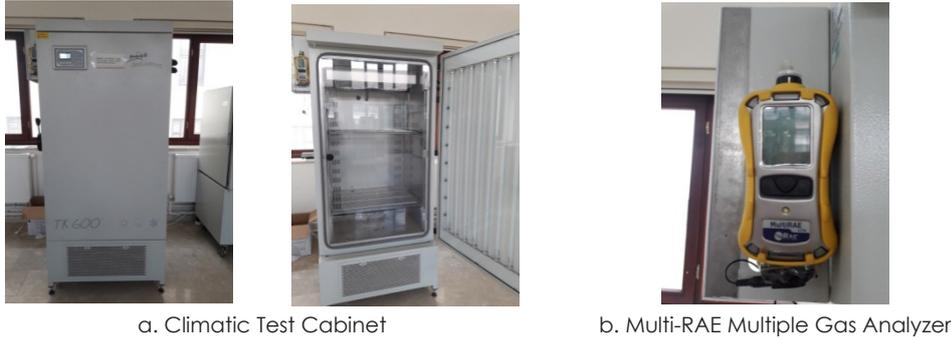
**Figure 2.a/b** Climatic test cabinet and Multi-RAE Multiple gas analyzer
