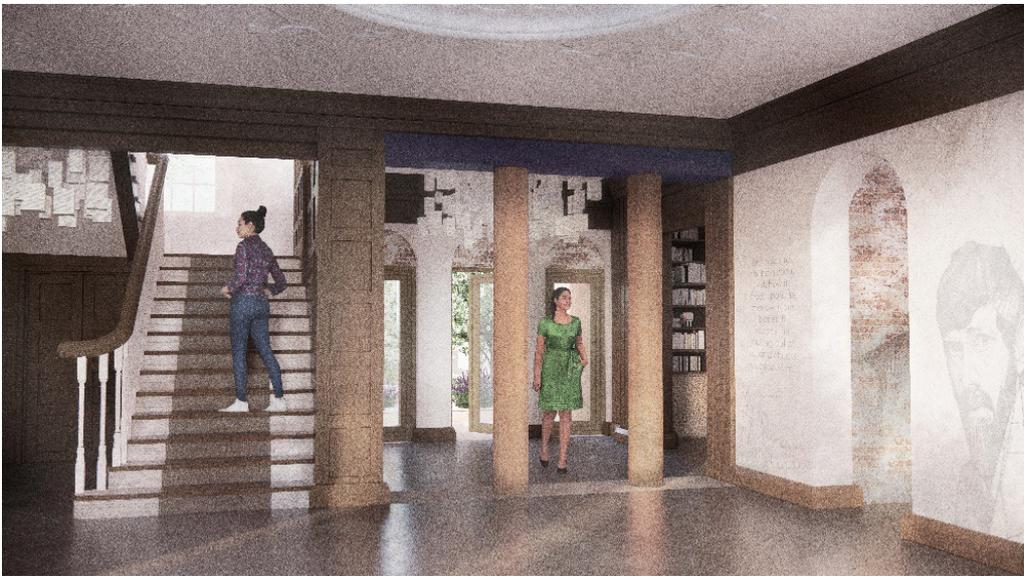
**Figure 32.** County House's original entrance chamber retains as much of the existing fabric as possible but balances this with the need to make repairs and to rationalize the internal layout. Floor tiles, where damaged, are swapped with travertine replacements formed using crushed brick from nearby demolition works, while traces remain of the timber Victorian staircase, removed and fitted elsewhere. New doors in the place of windows are picked out in brass, as are structural interventions.
